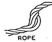
Fig. 17. ROPE DEFORMATION BY KINKING
